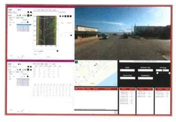
detection of cracks, lane-markings, man-made objects, and other distresses. The detected cracks are overlaid on the pavement images and offset to assist with the verification of the detected cracks. During reporting, the distress cracks are defined by road zone and accumulated according to the units defined in the client specification. The severity levels are identified based on the defined limits (ASTM D6433) and verified for resolution through visual quality control checks of image files.
